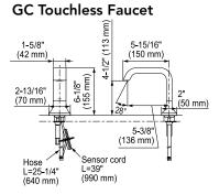
■Mounting deck thickness: 1/4" (5 mm) - 2" (50 mm) ■Spout hole: Ø1-1/4" (Ø32 mm) - Ø1-3/8" (Ø35 mm)
